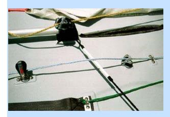
To keep the spinnaker halyard from re-cleating simply tie some bungee cord from the center bar to the outer bar. The bungee keeps the spinnaker halyard up and out of the reaches of the cleat during take down. In the photo this set-up has a plastic tube to protect the bungee from the friction of the halyard. It is simply taped in place.
