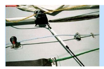
To keep the spinnaker halyard slack neat and out of the way use a thin diameter bungee and 2 small blocks. As you look at the photo you see that one block is TIED to the rear of the hiking strap eyelet.
